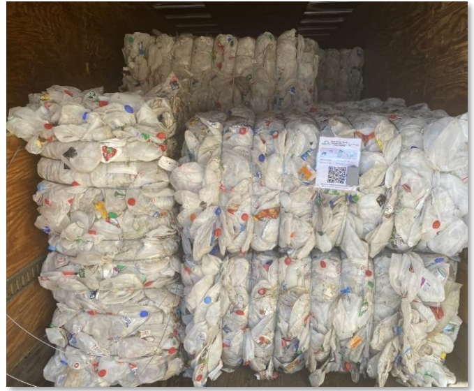
Photo 2: Bales of HDPE seen on the trailer at GreenWaste MRF before departure to Processor. Kamilo's QR & GPS identifiers used to track the shipment can be seen on the last bale. February 10, 2022.
