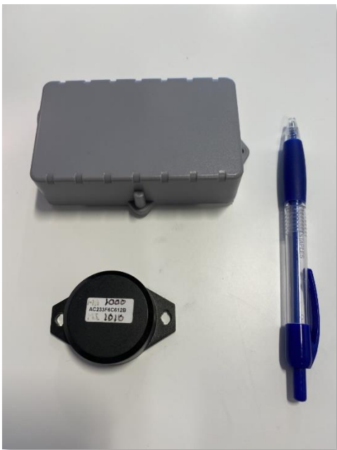
Photo 3: 2 Types of electronic transponders used for Pilot: GPS (top) and Bluetooth Low Energy (bottom).
